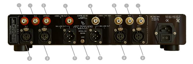
(1) **UNBALANCED INPUTS:** If you are using unbalanced RCA interconnects from your source components (CD player, tuner, etc.), they should be connected to unbalanced INPUTS 1 and If you have had the optional phono section card installed in the CAPRI S2-SC PREAMPLIFIER, the interconnects from the turntable or digital source should be installed into INPUT 1. For more information about the phono options, please contact your dealer.
