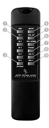
(9) **BAL R:** This button will shift the output of the preamplifier towards the right channel. Each press of the button will increase the output of right channel by 0.5 dB and decrease the level of the left channel by 0.5 dB. A total shift of 6 dB is possible. The balance control is not continuous; holding the button down will not continue to shift the balance. The button must be repeatedly pressed to continue to activate the balance shift towards the right channel.
