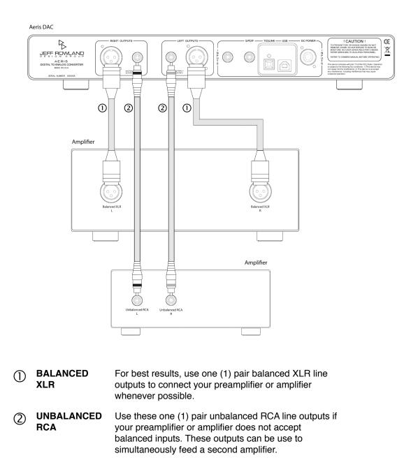
**NOTE**: The output levels of each pair of outputs are equivalent. It is unnecessary to compensate for a 6dB loss when using the RCA outputs.
