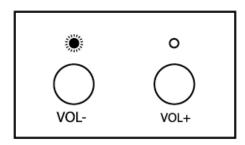
FLASHING LEFT LED Indicates unit volume is less than -32 dB.
