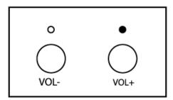
**SOLID RIGHT LED/NO LEFT LED** Indicates maximum volume level with no potential loss of resolution.
