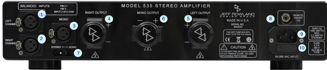
Figure 2: Rear Panel Connections
