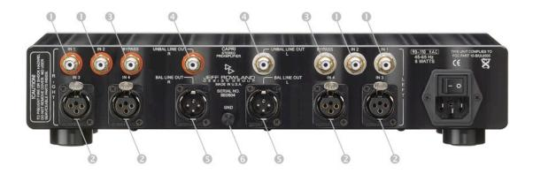
(1) UNBALANCED INPUTS: If you are using unbalanced RCA interconnects from your source components (CD player, tuner, etc.), they should be connected to unbalanced INPUTS 1 and If you have had the optional phono section or DAC card installed in the CAPRI S2 PREAMPLIFIER, the interconnects from the turntable or digital source should be installed into INPUT 1. For more information about the phono option or DAC option, please contact your dealer.
